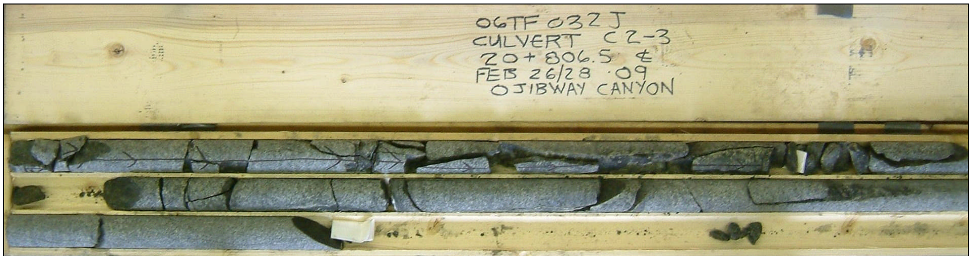
Photograph 2: Culvert C8, borehole C8-3, RC-7 to RC-9. RQD ranged from 15 to 100%. Rock quality ranged from very poor to excellent.
