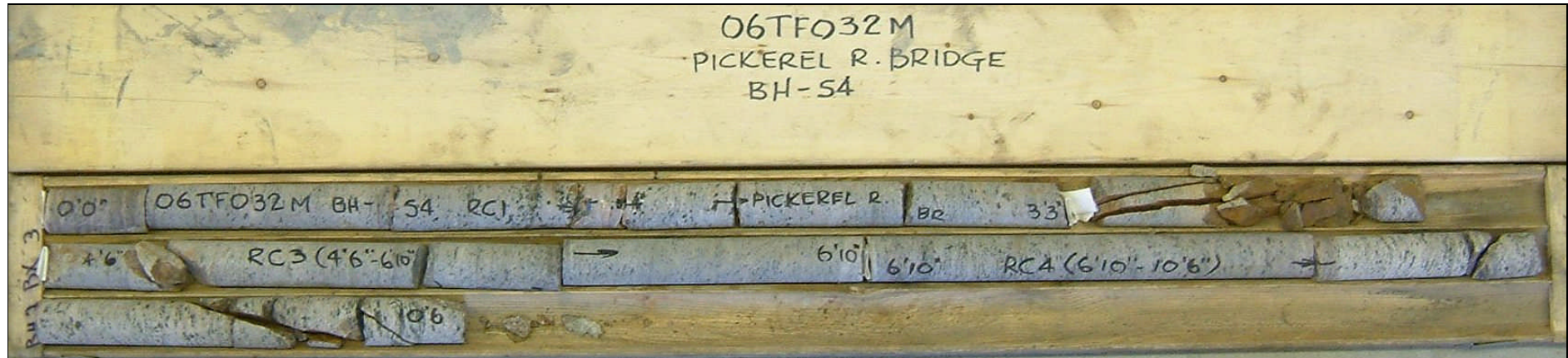
Photograph 3: Borehole S4, samples RC-1 to RC-4 from 0.0 to 3.2 m depth. The RQD values ranged from 0 to 100%, indicating good to excellent (locally very poor) quality bedrock.
