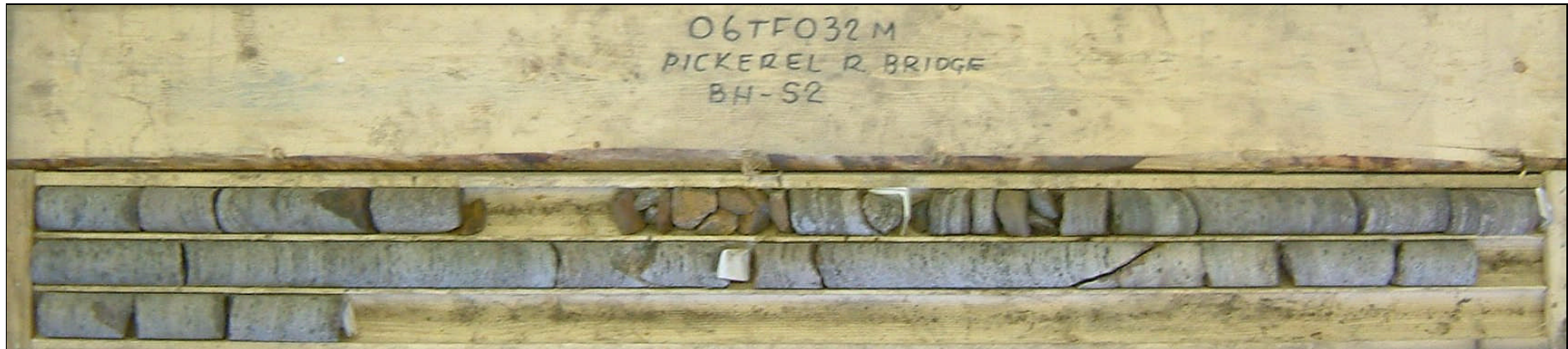
Photograph 1: Borehole S2, samples RC-1 to RC-4 from 0.0 to 3.1 m depth. The RQD values ranged from 31 to 96%, indicating poor becoming good to excellent quality bedrock.
