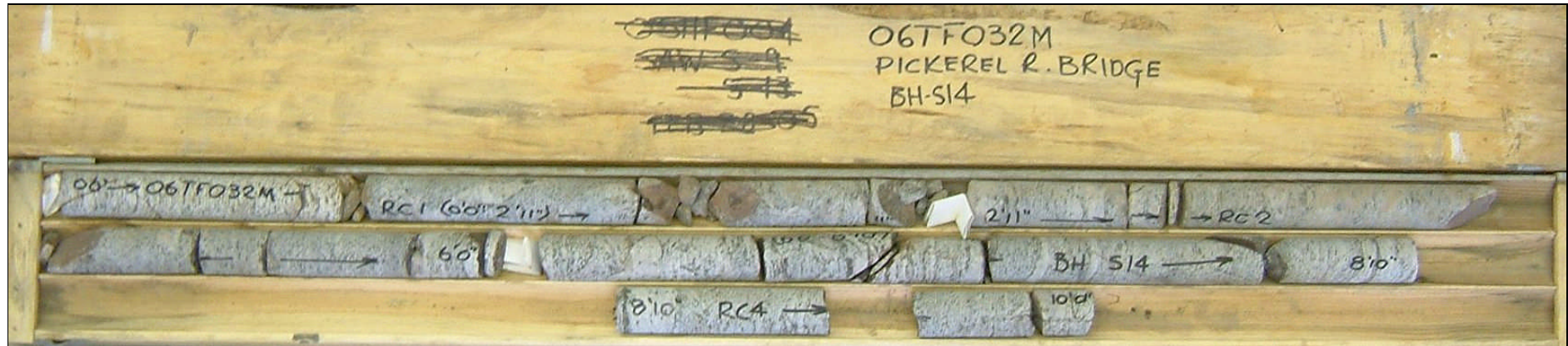
Photograph 9: Borehole S14, samples RC-1 to RC-4 from 0.0 to 3.1 m depth. The RQD values ranged from 0 to 94%, indicating excellent to fair becoming very poor quality bedrock.
