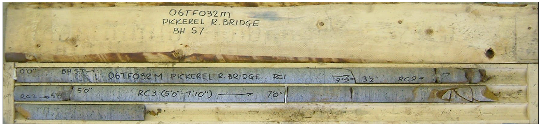
Photograph 4: Borehole S7, samples RC-1 to RC-4 from 0.0 to 3.1 m depth. The RQD values ranged from 59 to 100%, indicating fair to excellent quality bedrock.
