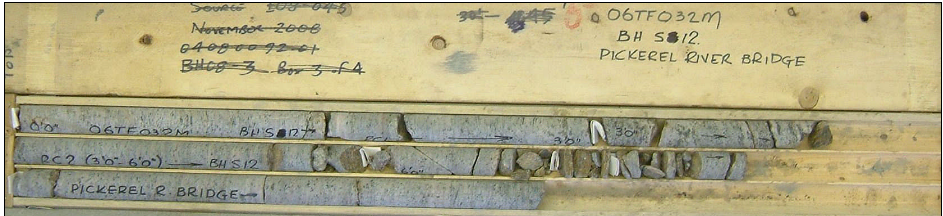
Photograph 7: Borehole S12, samples RC-1 to RC-6 from 0.0 to 3.1 m depth. The RQD values ranged from 0 to 99%, indicating fair to excellent (locally very poor) quality bedrock.
