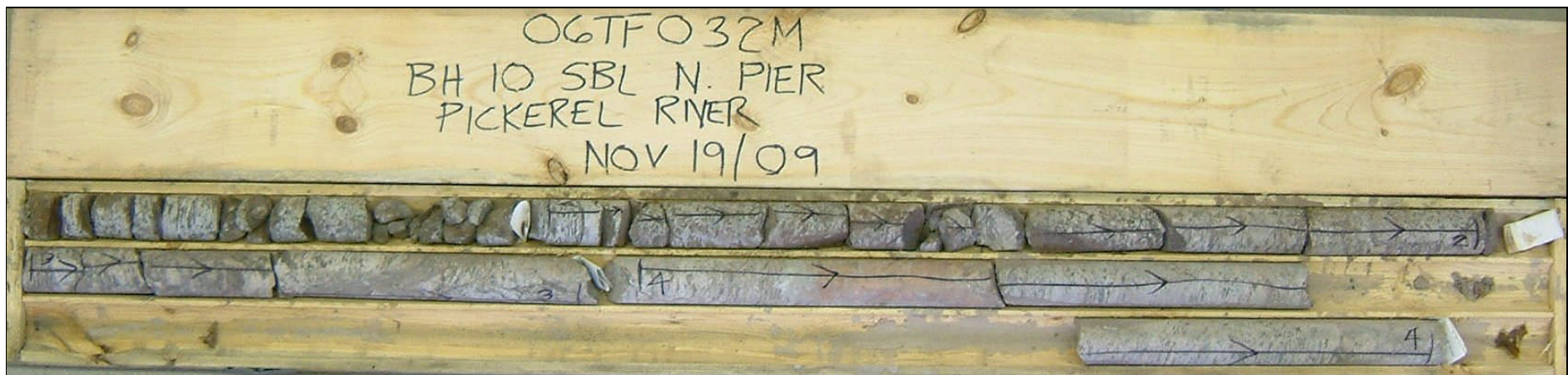
Photograph 12: Borehole S19, samples RC-1 to RC-4 from 0.0 to 3.1 m depth. The RQD values ranged from 0 to 95%, indicating very poor to poor becoming good to excellent quality bedrock.
