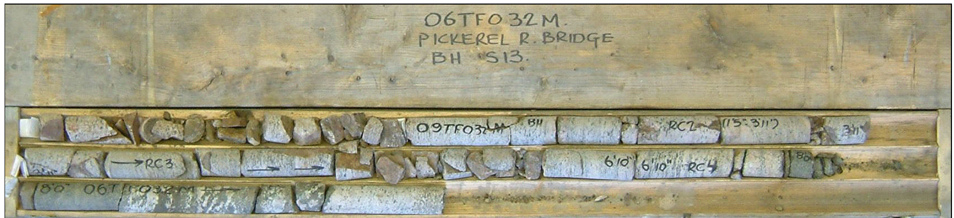
Photograph 8: Borehole S13, samples RC-1 to RC-5 from 0.0 to 3.2 m depth. The RQD values ranged from 0 to 83%, indicating very poor to poor becoming good quality bedrock.
