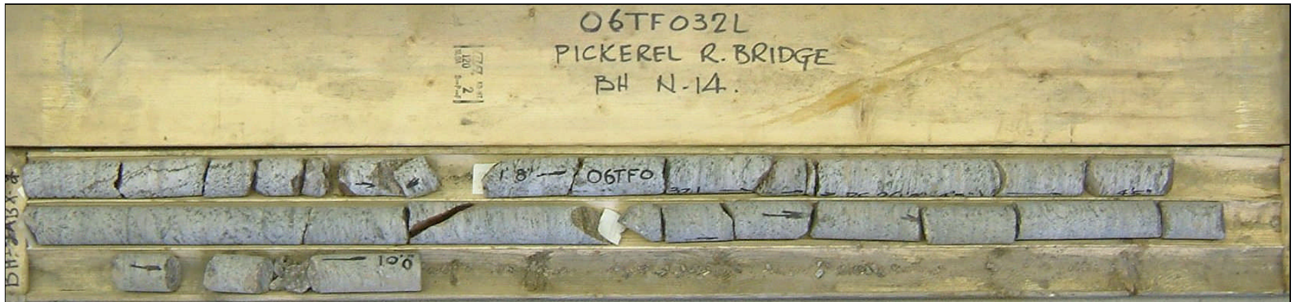
Photograph 9: Borehole N14, samples RC-1 to RC-4 from 0.0 to 3.1 m depth. The RQD values ranged from 40 to 88%, indicating poor becoming fair to good quality bedrock.
