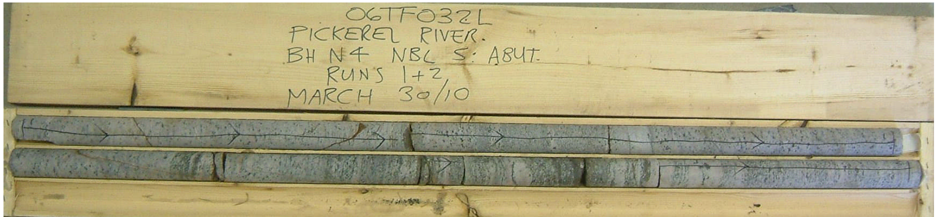
Photograph 2: Borehole N4, samples RC-1 and RC-2 from 0.4 to 3.4 m depth. The RQD values were 94 and 100%, indicating excellent quality bedrock.
