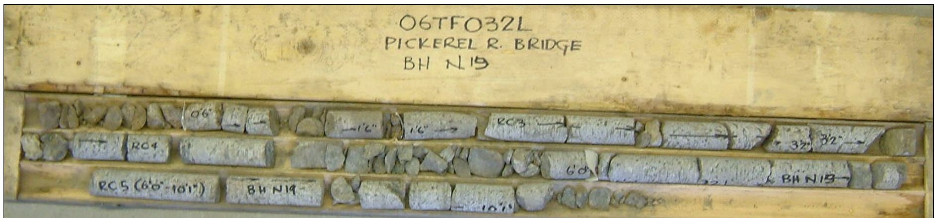
Photograph 12: Borehole N19, samples RC-1 to RC-5 from 0.0 to 3.1 m depth. The RQD values ranged from 0 to 80%, indicating very poor becoming fair to good (locally poor) quality bedrock.
