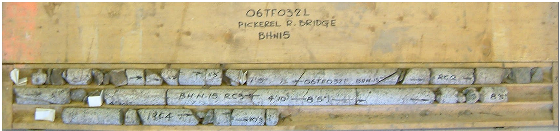
Photograph 10: Borehole N15, samples RC-1 to RC-4 from 0.0 to 3.1 m depth. The RQD values ranged from 0 to 93%, indicating very poor becoming fair (locally excellent) quality bedrock.
