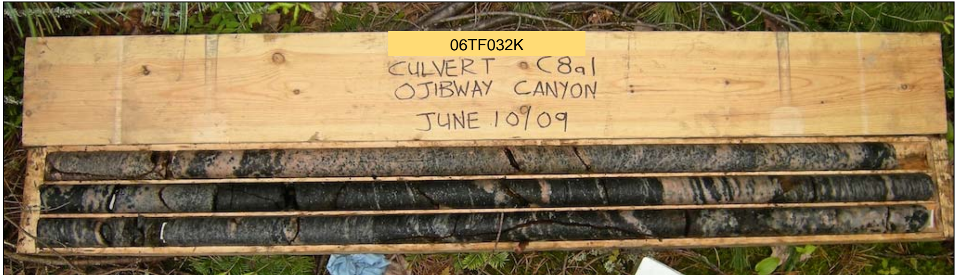
Photograph 1: Culvert C8a, borehole C8a-1, samples RC-1 to RC-3. The RQD value ranged from 41 to 97%. Rock quality ranged from poor to fair becoming excellent.
