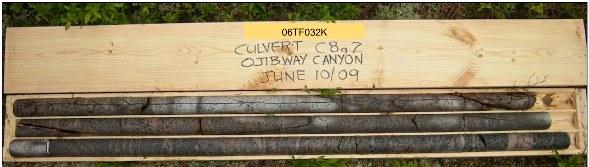
Photograph 2: Culvert C8a, borehole C8a-2, samples RC-1 to RC-3. The RQD value ranged from 59 to 100%. Rock quality ranged from fair to excellent.
