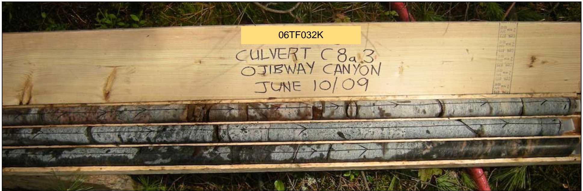
Photograph 3: Culvert C8a, borehole C8a-3, samples RC-1 to RC-3. The RQD value ranged from 79 to 100%. Rock quality ranged from good to excellent.
