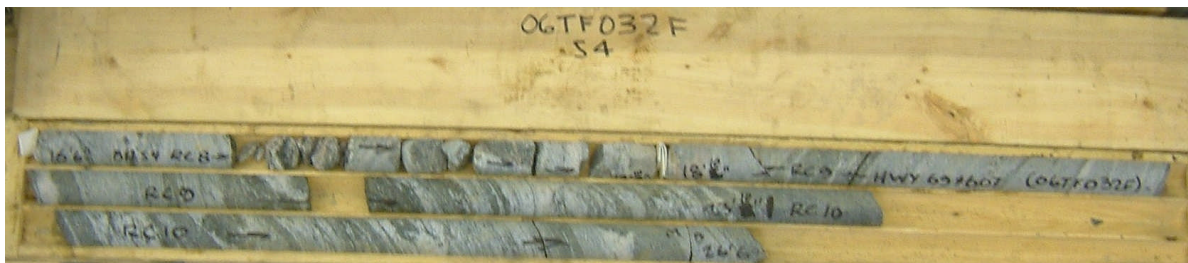
Photograph 3: Cores retrieved from Borehole S4. Runs 8 to 10 from 5.0 to 8.1 m depth. RQD ranged from 54 to 100%. Upper 0.7 m rock, from 5.0 to 5.7 m depth, is fair quality, remainder excellent quality.
