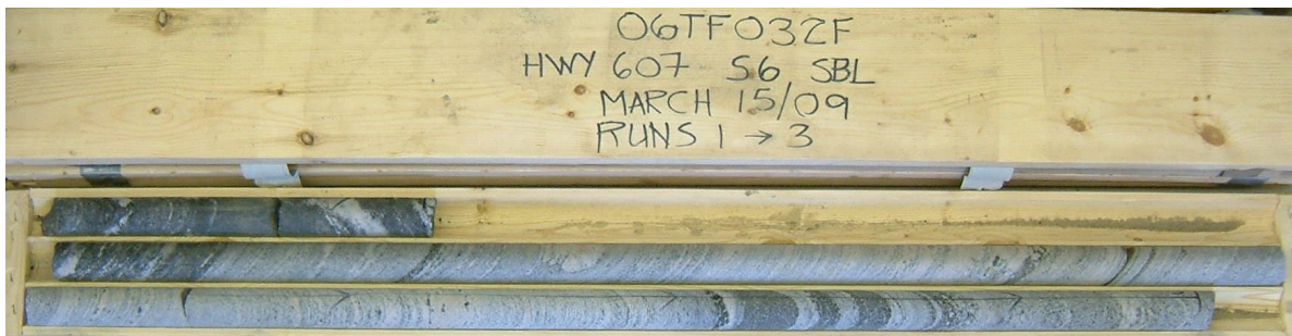
Photograph 5: Cores retrieved from Borehole S6. Runs 7 to 9 from depth 3.4 to 6.8 m. Last 7.5 cm rock piece remained down hole. RQD ranged from 95 to 100%, excellent quality.
