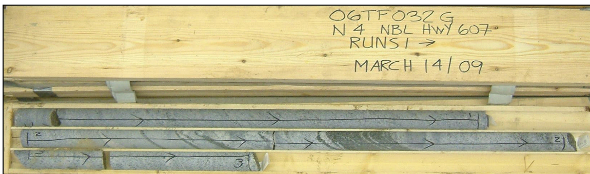
Photograph 2: Cores retrieved from Borehole N4. Runs 2 to 4.
