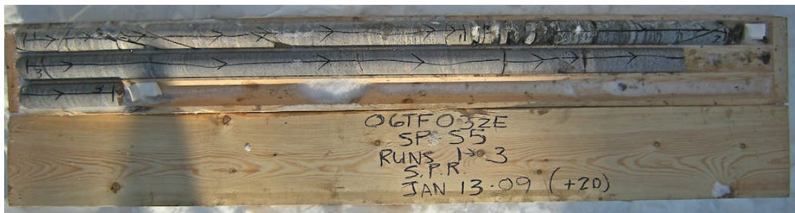
Photograph 3: Rock cores retrieved from borehole SP-S5. Samples RC-8 to RC-10.
