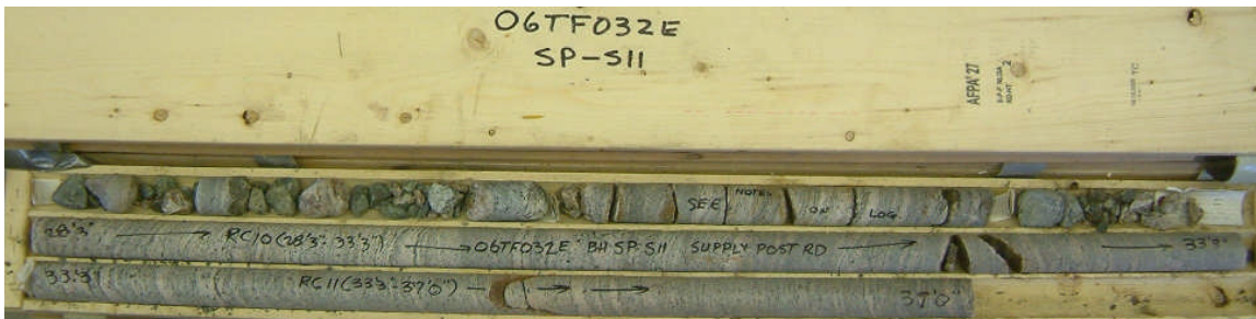
Photograph 7: Rock cores retrieved from borehole SP-S11. Samples RC-8 to RC-11.
