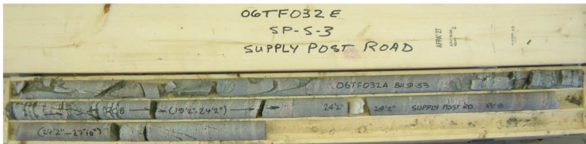
Photograph 1: Rock cores retrieved from borehole SP-S3. Samples RC-7 to RC-9.
