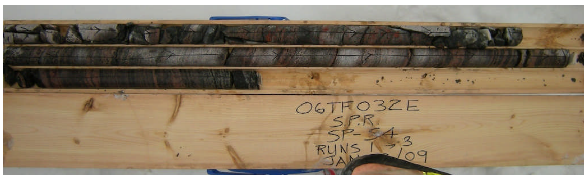
Photograph 2: Rock cores retrieved from borehole SP-S4. Samples RC-10 to RC-12.
