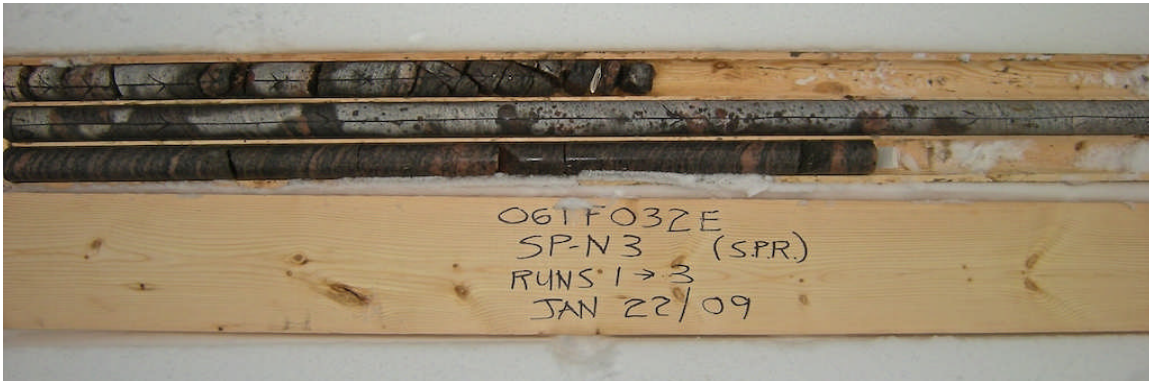
Photograph 1: Rock cores retrieved from borehole SP-N3. Samples RC-2 to RC-4.
