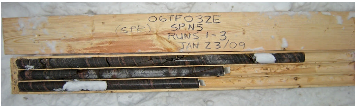
Photograph 3: Rock cores retrieved from borehole SP-N5. Samples RC-1 to RC-3.
