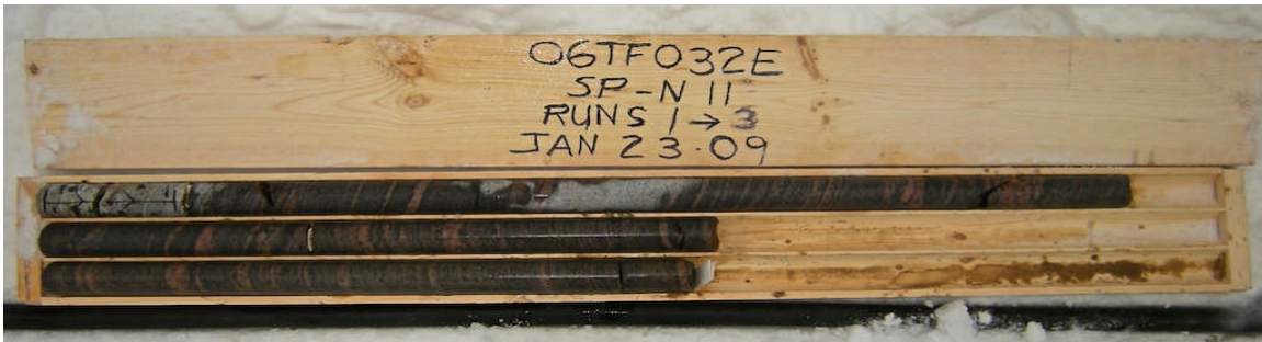
Photograph 7: Rock cores retrieved from borehole SP-N11. Samples RC-2 to RC-4.
