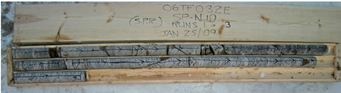
Photograph 6: Rock cores retrieved from borehole SP-N10. Samples RC-3 to RC-5.
