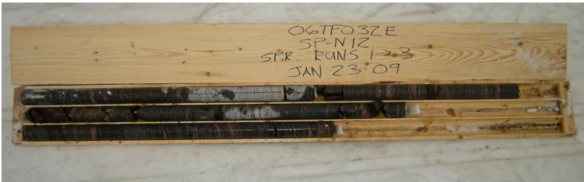
Photograph 8: Rock cores retrieved from borehole SP-N12. Sample RC-1 to RC-3.
