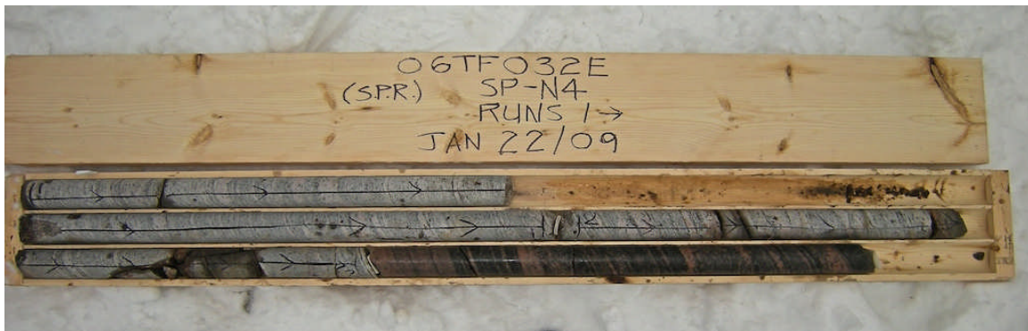
Photograph 2: Rock cores retrieved from borehole SP-N4. Samples RC-1 to RC-3.
