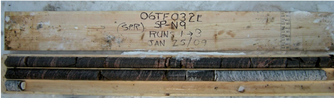
Photograph 5: Rock cores retrieved from borehole SP-N9. Samples RC-3 to RC-5.
