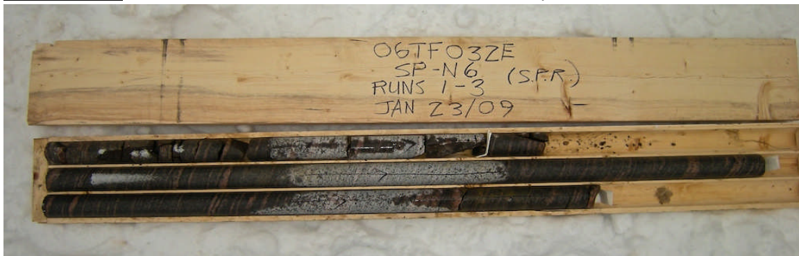
Photograph 4: Rock cores retrieved from borehole SP-N6. Samples RC-1 to RC-3.
