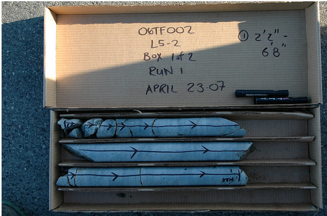
Photograph 7: Rock cores from L5-2, Run 1.
