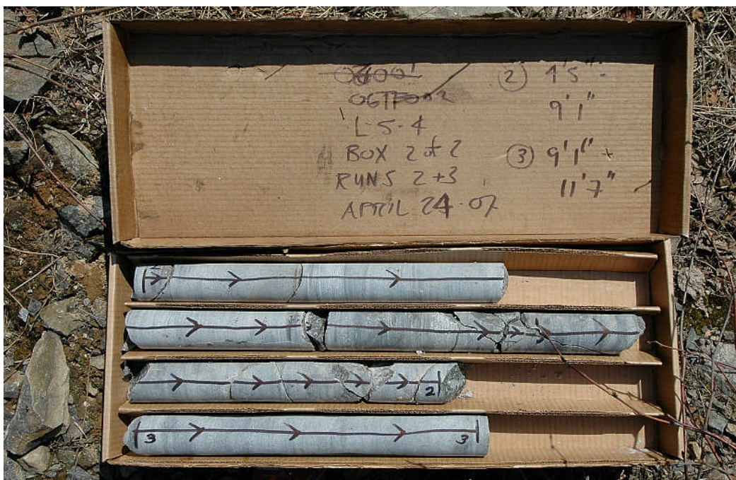
Photograph 12: Rock cores from L5-4, Runs 2 and 3.
