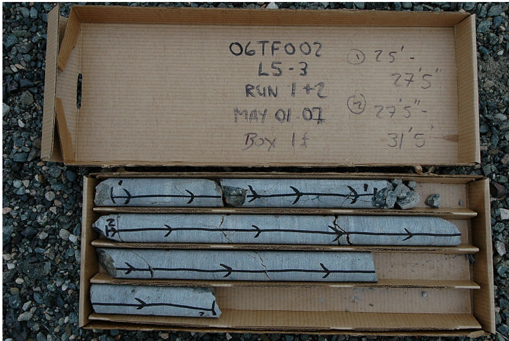
Photograph 9: Rock cores from L5-3, Runs 1 and 2.
