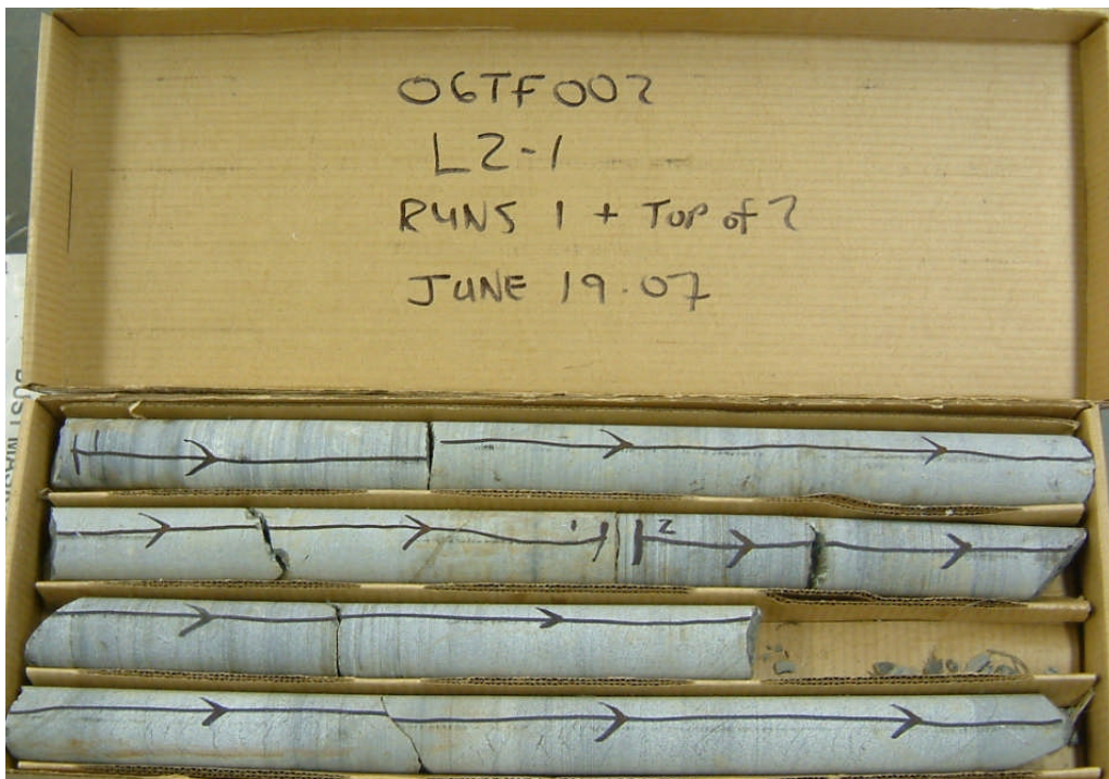
Photograph 1: Arkose rock core from borehole L2-1, RC-18 and RC-19. (RQD 100% for both runs)
