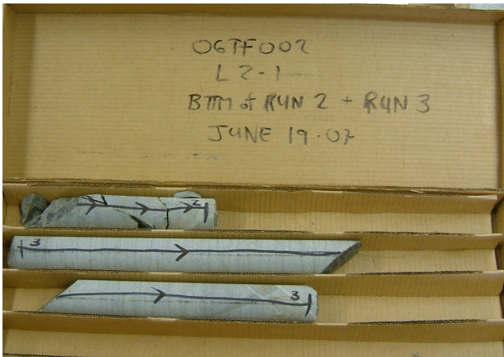
Photograph 2: Arkose rock core from borehole L2-1, RC-19 and RC-20. (RQD 100% for both runs)
