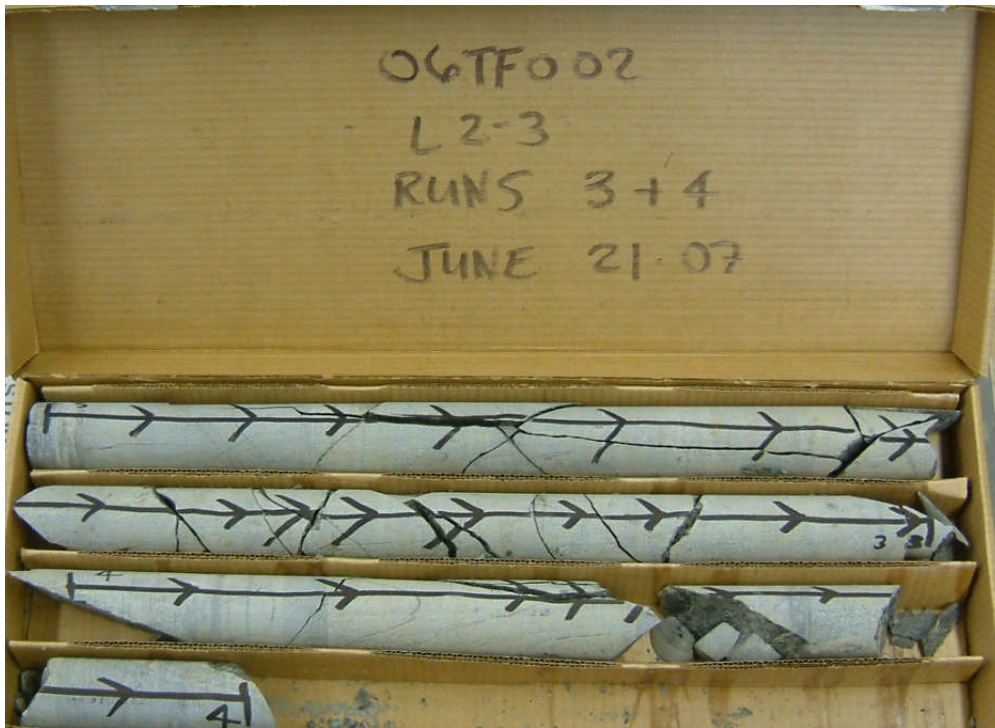
Photograph 5: Argillite rock core from borehole L2-3, RC-22 and RC-23. RQD values of 65 and 100%.
