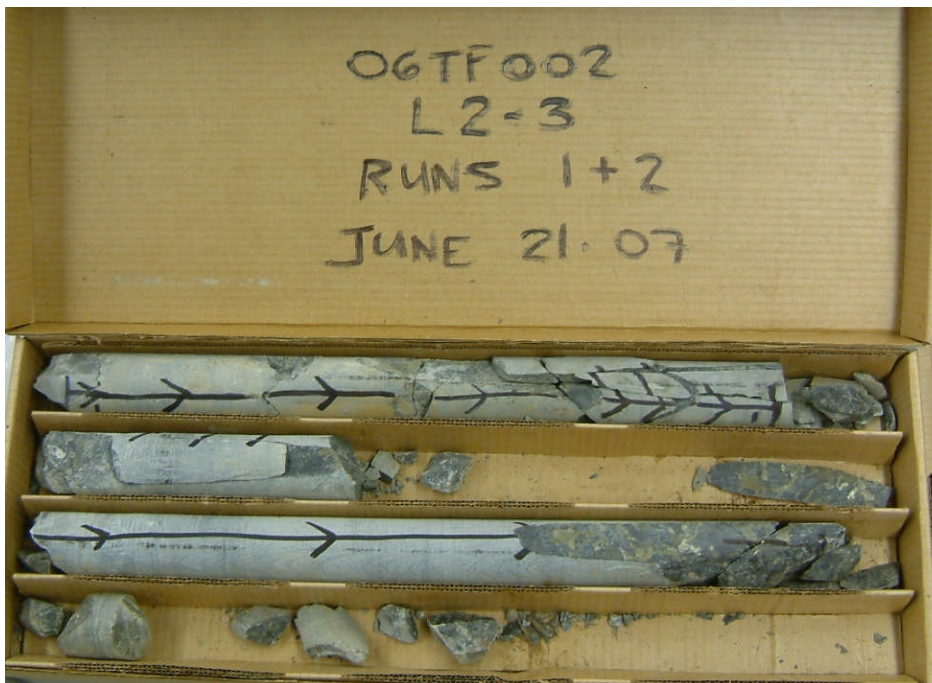
Photograph 4: Argillite rock core from borehole L2-3, RC-20 and RC-21. RQD values of 54 and 90%.
