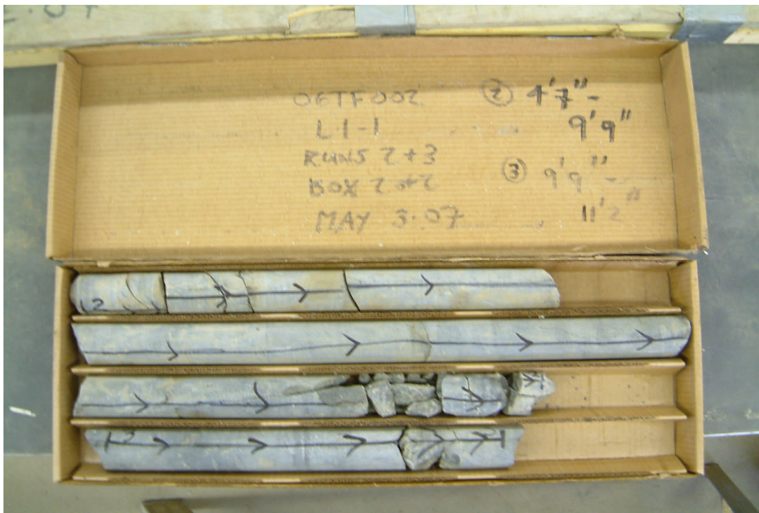
Photograph 2: Argillite rock core from borehole L1-1, RC-2 and RC-3. RQD values of 65 and 100% for RC-2 and RC-3, respectively.
