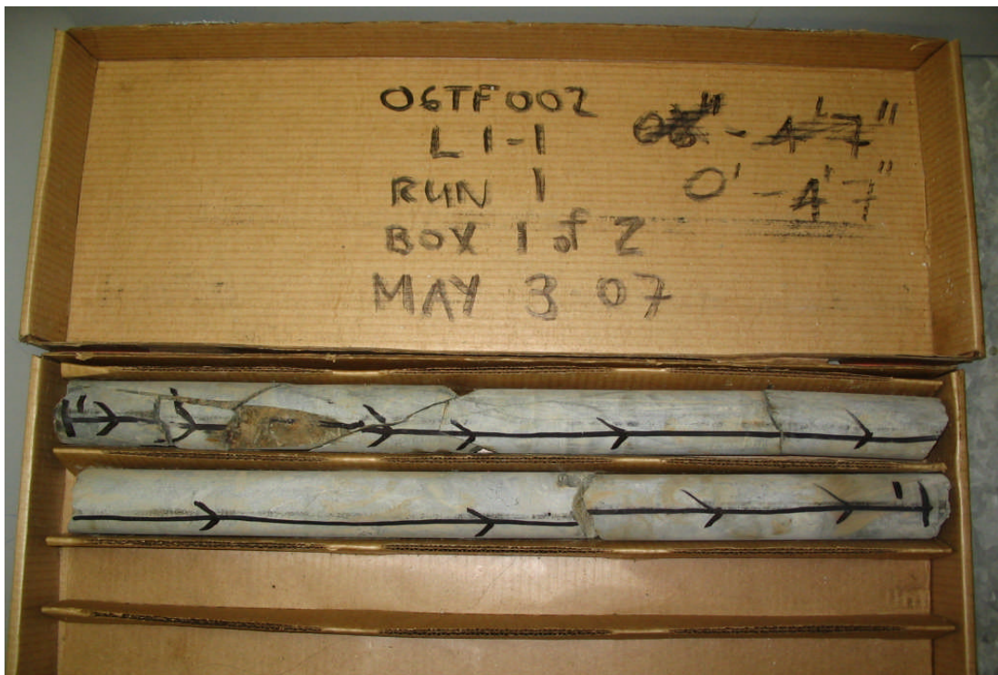
Photograph 1: Argillite rock core from borehole L1-1, RC-1. RQD value of 75%.
