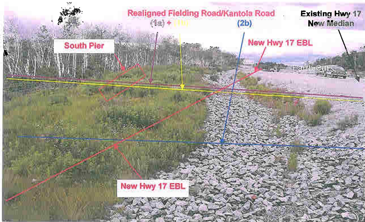
Photograph 56 VIEW: Looking west from west shoulder of Kantola Road at Highway 17 south ditch line. No bedrock exposure in view. Existing 6 m high earth slopes with stone riprap at STA. 16+800 visible in distance. (July 5, 2006)
