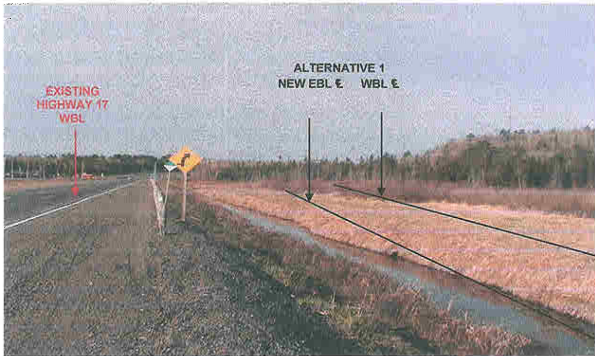
Photograph 3 VIEW: Highway 17 Sta. 17+700 (Alt. 1). Looking westerly from north shoulder of westbound lanes. Note ditch and swamp beyond embankment. Alternatives 2 and 3 (not shown) are located between Alternative 1 and existing Highway WBL. Depth to bedrock is over 24 m, about 15 m to firm bottom in Fairbank Creek floodplain. (May 1, 2006)
