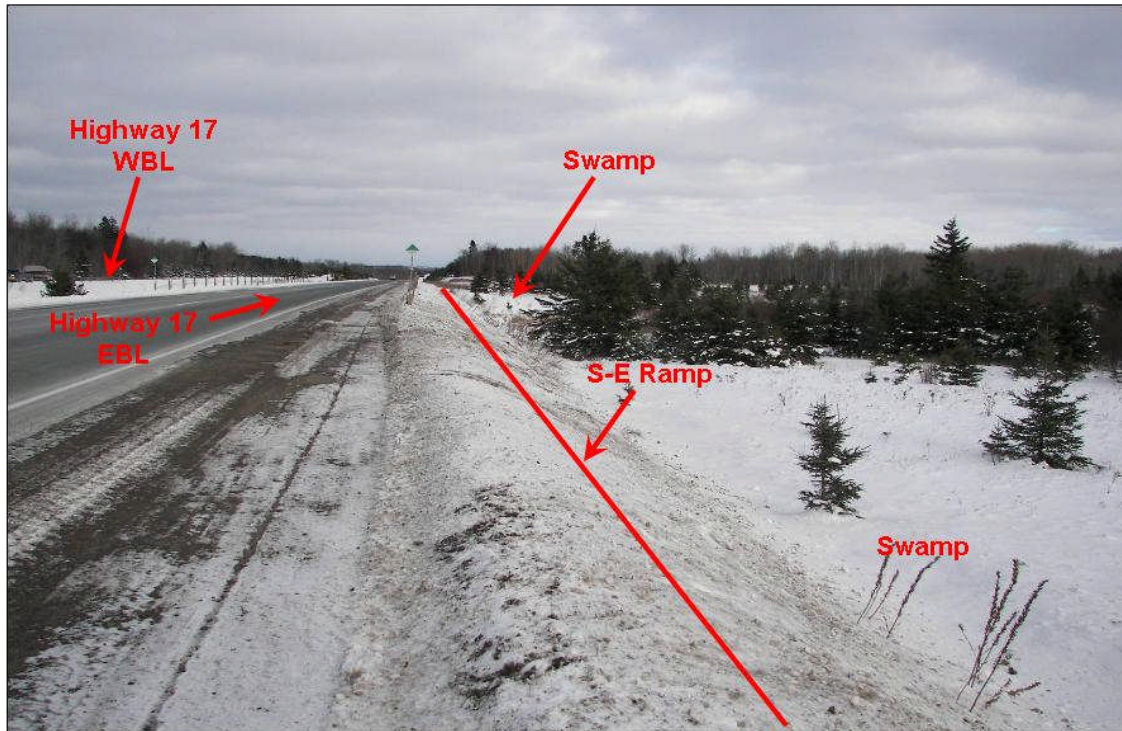
Photograph 125 VIEW: Looking east from south shoulder of Highway 17 EBL about 1,050 m east of existing SMR3 underpass. Note low-lying swampy ground to the south where S-E ramp construction will require widening of the highway embankment. (Dec. 6, 2007)
