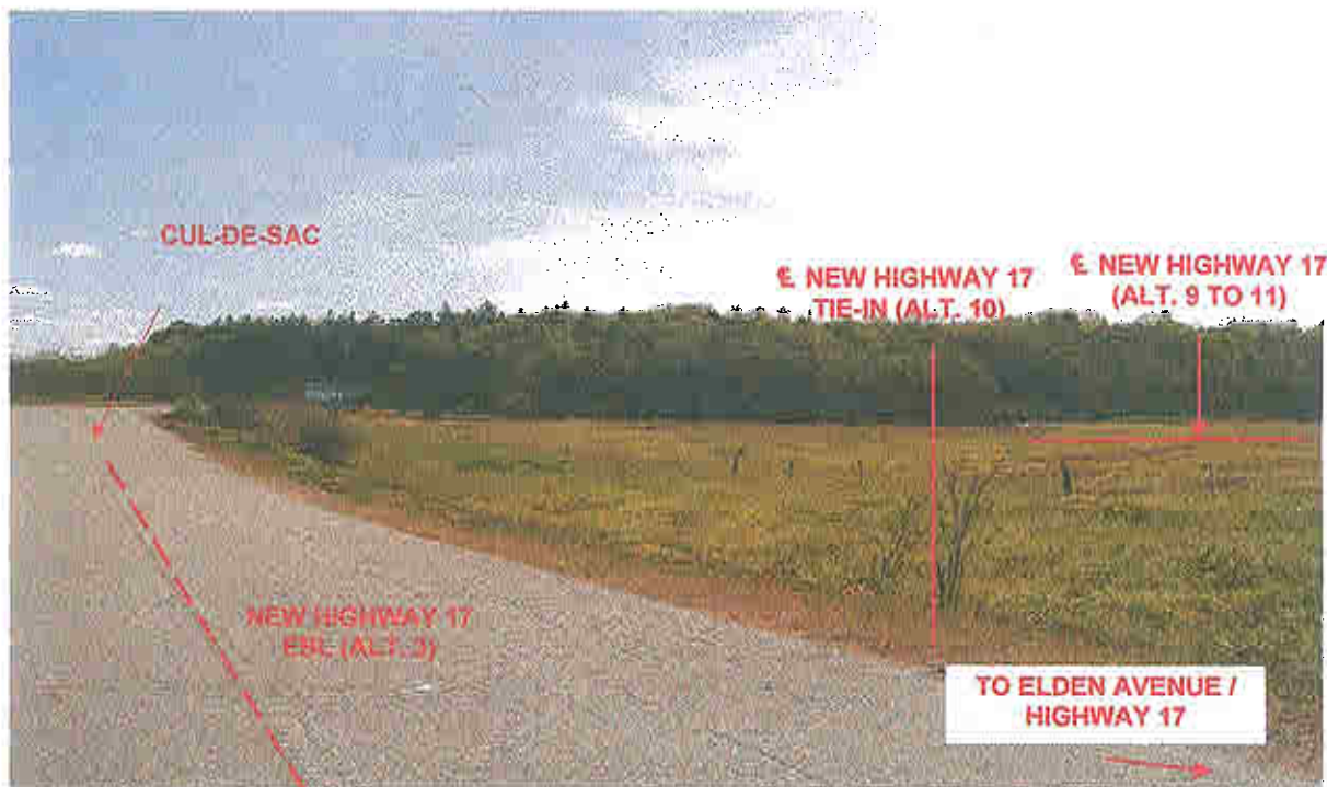
Photograph 32 VIEW: Looking southeast from roadway to cul-de-sac off Elden Avenue south of Highway 17. New Highway 17 EBL centreline (Alt 3) to left of photograph. Tie-in for Alt. 10 to centre right. Alignment for Alt. 9 to 11 in distance right. Flat open field to rolling terrain at bush line. Massive rock outcrop on M. Rocha property in distance. (August 2005)
