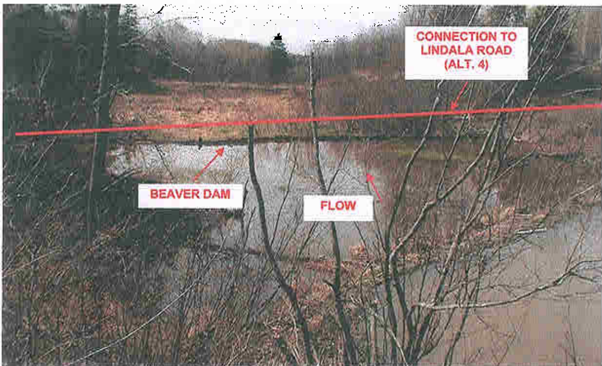
Photograph 22 VIEW: Looking south across pond of beaver dam immediately north of potential connecting road from St. Pothier Road to Lindala Road, approximately south of Sta. 17+050 (Alt. 4). Swamp crossing is about 40 m wide, culvert required. (May 1, 2006)
