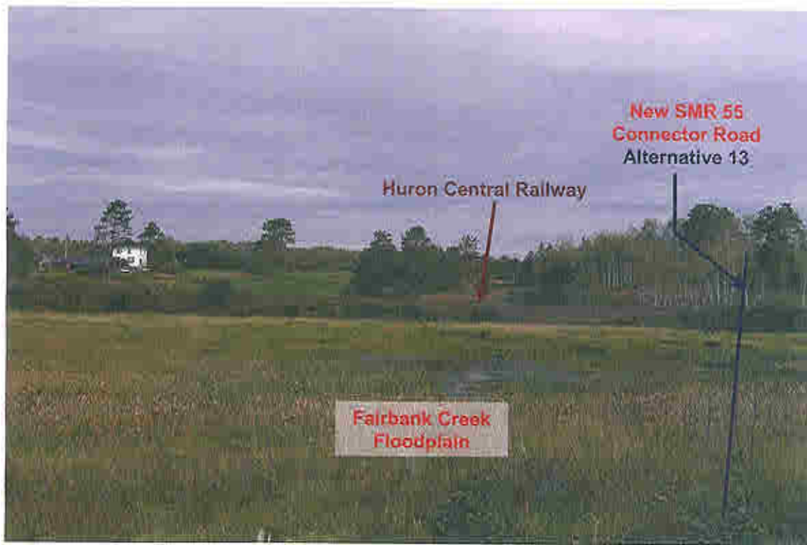
Photograph 91 VIEW: Looking northeast across Fairbank Creek Floodplain about 150 m east of SMR 55. Estimated depth 10 to 12 m to "firm bottom". (September 12, 2006)
