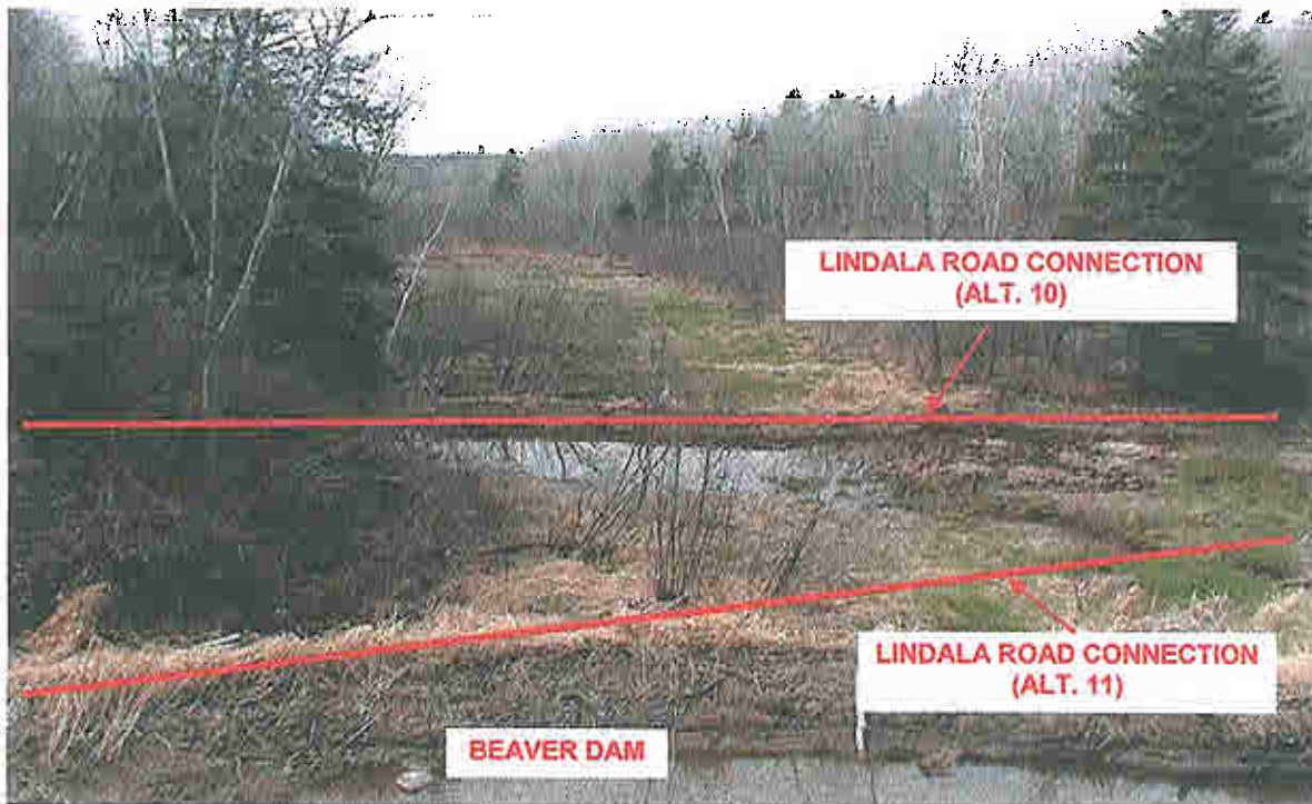
Photograph 23 VIEW: Looking south at connecting roads to Lindala Road for Alternatives 10 and 11 through swamp and creek of Rocha's land. Swamp is about 40 m wide. Culverts are required. (May 1, 2006)
