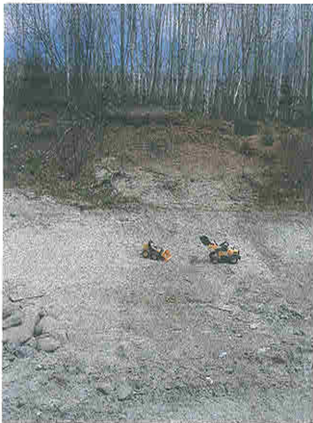
Photograph 27 VIEW: Looking east at exposed 2 m overburden slope at rear of M. Rocha residence, 716 St. Pothier Road. Soil profile comprised upper 1 m of reddish brown fine sandy silt over dense grey silt. (May 1, 2006)
