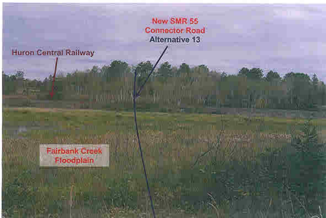
Photograph 92 VIEW: Looking east across Fairbank Creek Floodplain about 150 m east of SMR 55. Estimated depth 10 to 12 m to "firm bottom". (September 12, 2006)
