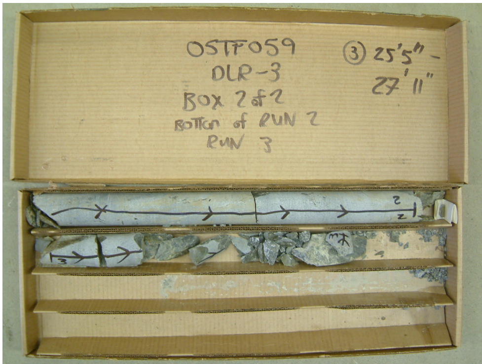
Photograph C-4: Rock core from borehole DLR-3. Bottom of samples RC7 and RC8. Note that bottom 0.4 m of sample RC8 could not be retrieved from the borehole.
