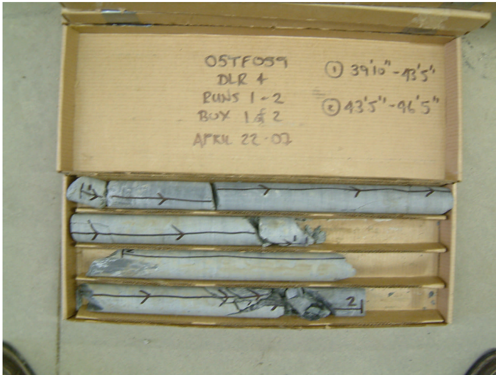
Photograph C-5: Rock core from borehole DLR-4. Samples RC10 and RC11.
