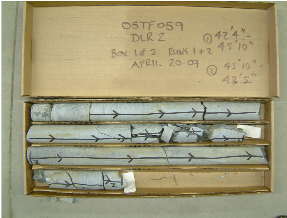
Photograph C-1: Rock core from borehole DLR-2. Samples RC6 and RC7.
