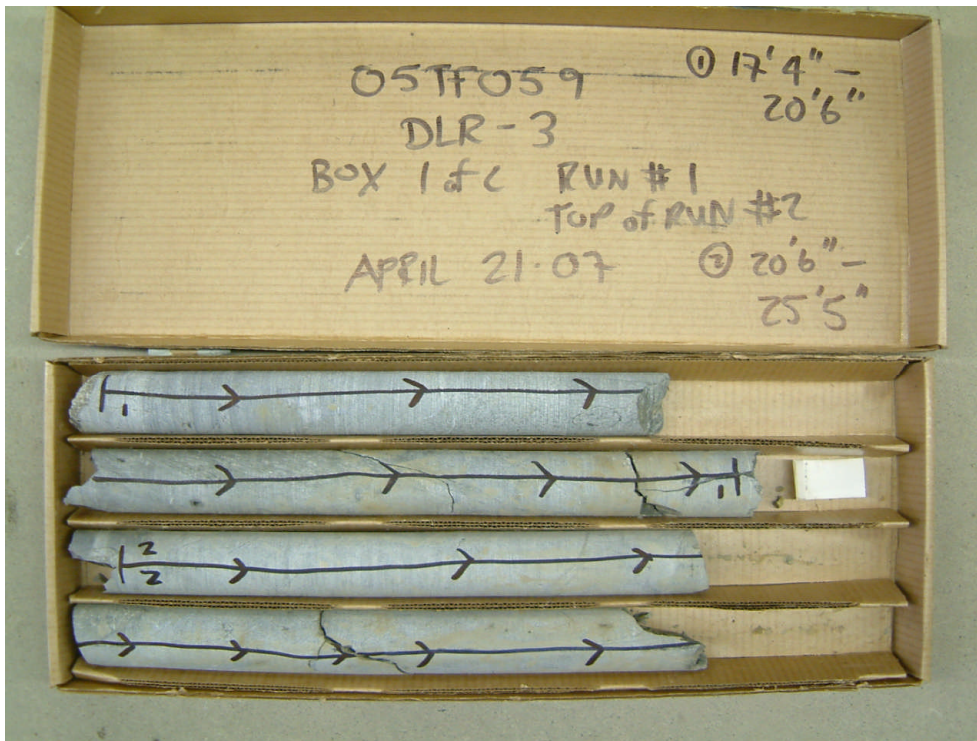
Photograph C-3: Rock core from borehole DLR-3. Samples RC6 and top of RC7.
