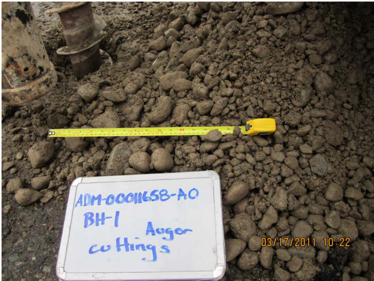
Photo No. 2: Auger cuttings from BH-1 consisting of sand and gravel fill with cobbles, that is underlain asphalt.
