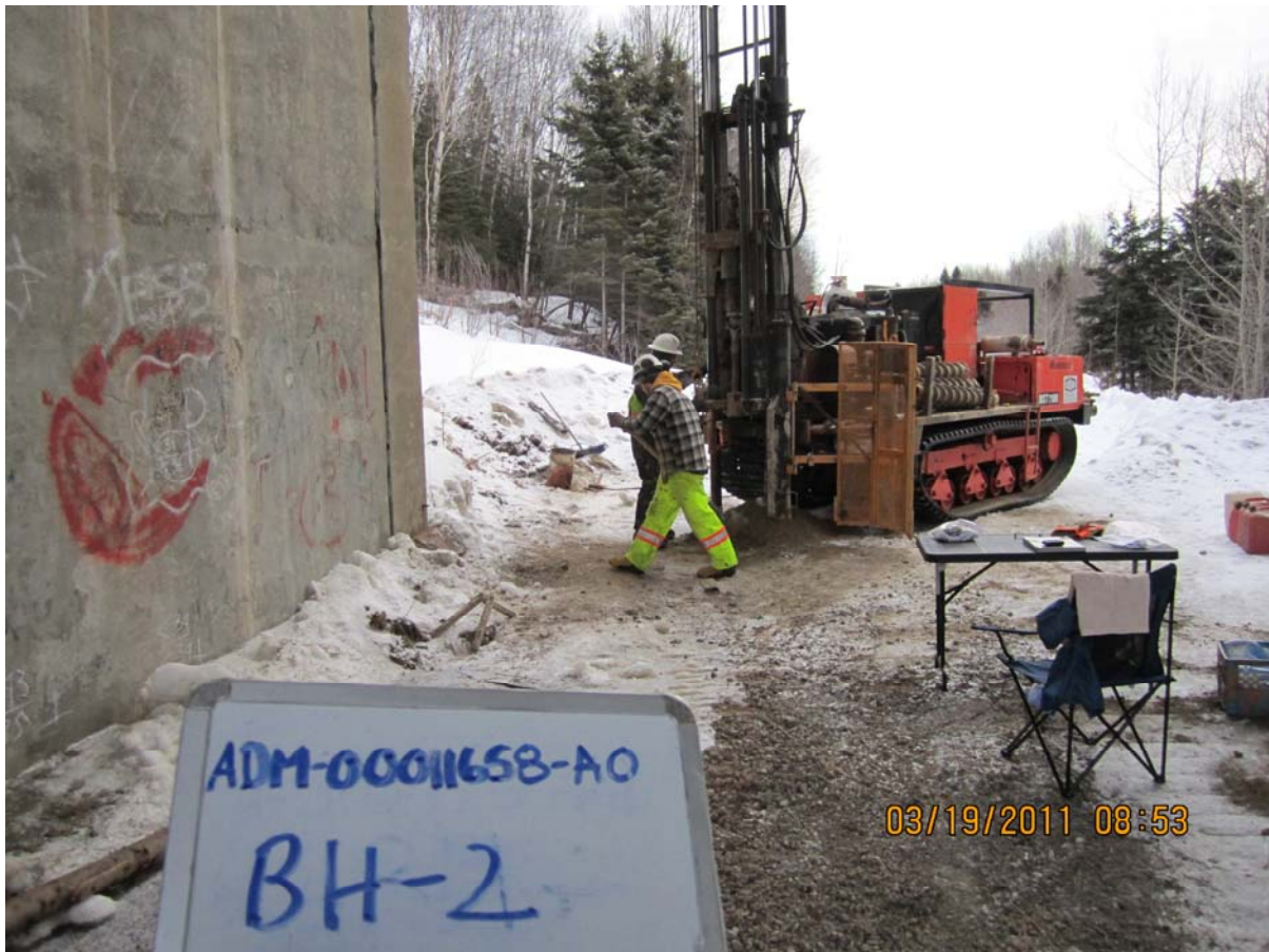
Photo No. 4: Set-up at BH-2 located on north-east side of bridge. Borehole advanced from historic railway surface. View looking north-east.
