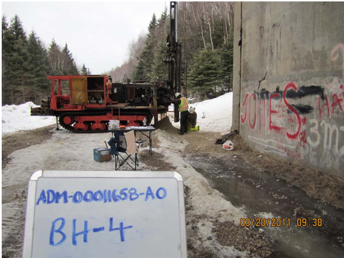
Photo No. 6: Set-up at BH-4 located on north-west side of bridge. Borehole advanced from historic railway surface. View looking north-west.
