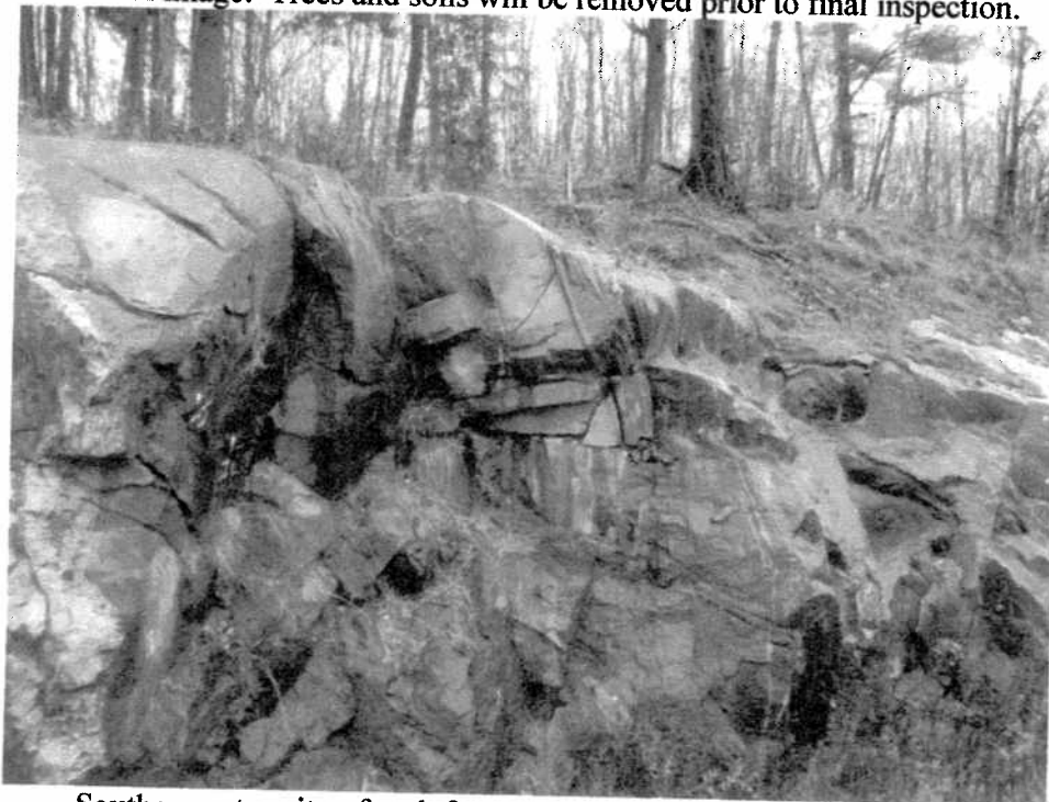
Image 4. Southern extremity of rock face under proposed abutment. Note fractured rock mass and curved, folded gneissic banding. Limited scaling will be needed to remove the loose rock from the face.
