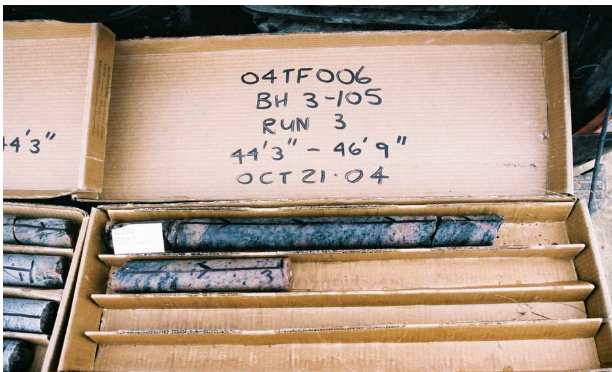
Plate 4. Granitic Gneiss Borehole 3-105, Rock Core 10 at Centre pier (South Mary Lake Road)
