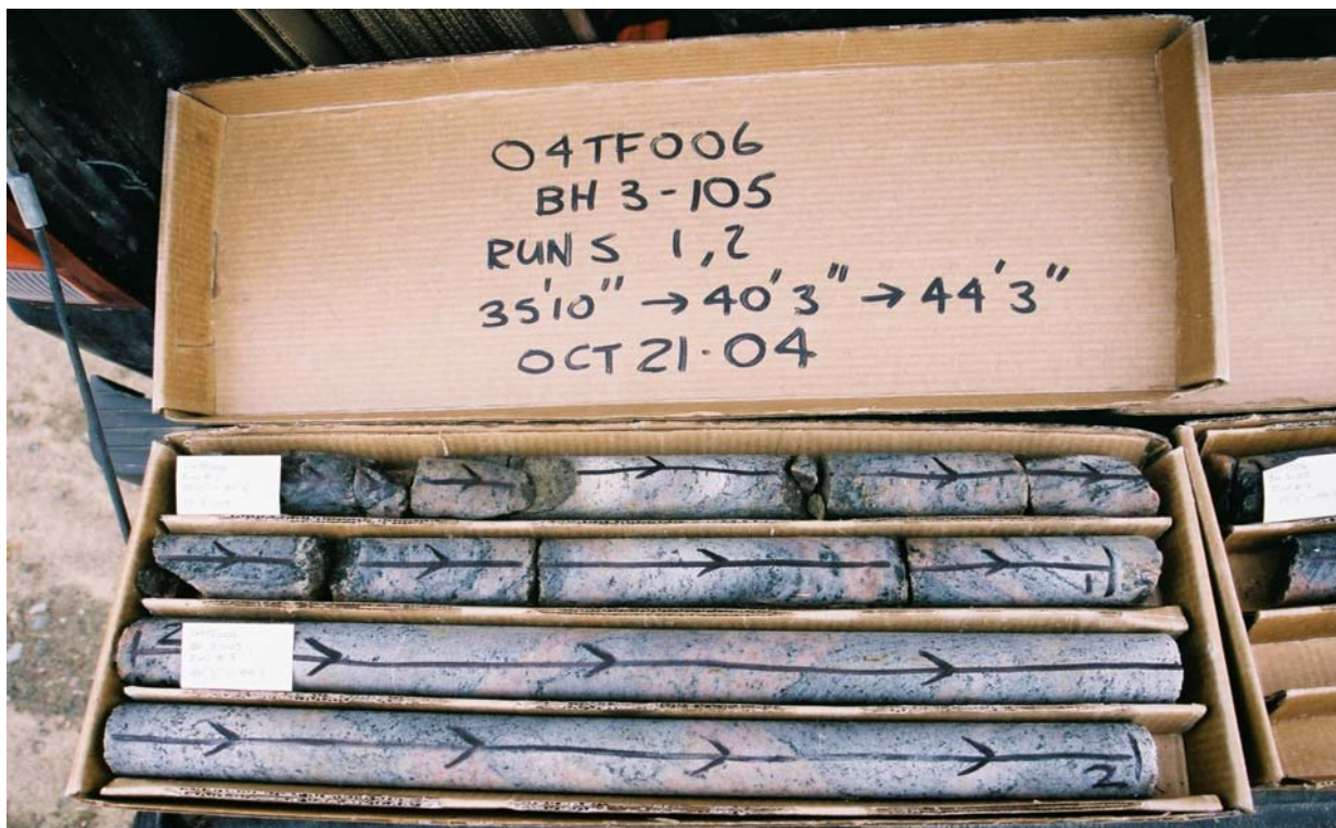
Plate 3. Granitic Gneiss Borehole 3-105, Rock Cores 8 and 9 at centre pier (South Mary Lake Road)
