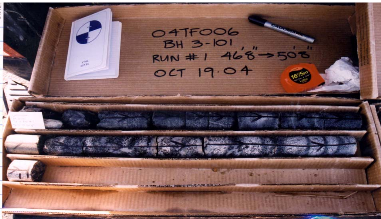
Plate 1. Biotite Gneiss Borehole 3-101, Rock Core 12 at west abutment (South Mary Lake Road)
