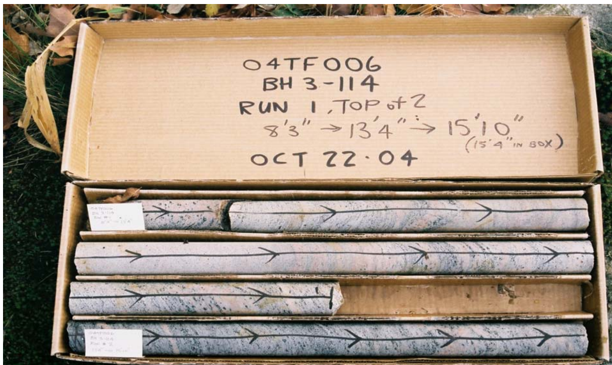
Plate 5. Granitic Gneiss Borehole 3-114, Rock Core 1 at east abutment (South Mary Lake Road)
