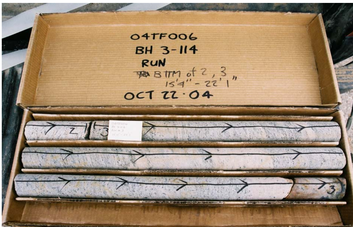
Plate 6. Granitic Gneiss Borehole 3-114, Rock Cores 2 and 3, at east abutment (South Mary Lake Road)
