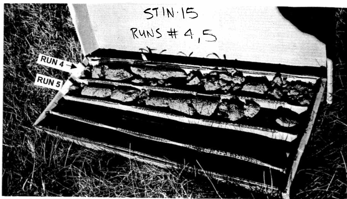
Plate No. 8: Core from Schist and granite bedrock taken from borehole ST1N-15 drilled at the location of the north pier.
